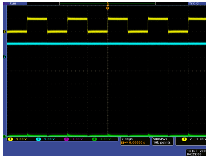
Figure 29. Functional behavior of competitor in Configuration 3 after test. CANH was stressed with +3 kV pulse and fails functional (bus levels and receiver).
